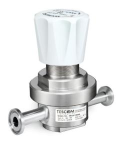
TESCOM PH-2600 Series is part of our Pharmpure™ product line. This high purity single-stage regulator offers a compact, USP Class VI and BPE compliant design suitable for specialty, corrosive, and pyrophoric applications. This regulator offers gas flows of <10 SCFM / 283 SLPM. Diffusion-resistant metal diaphragm seal ensures gas purity and integrity.
