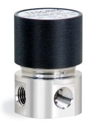
TESCOM BB-1 Series high pressure, low flow, miniature pressure reducing regulator provides six outlet pressure ranges available up to 1800 psig / 124 bar outlet. This non-venting regulator is small and compact, weighing approximately 0.5 lbs / 0.2 kg in the standard aluminum construction.
