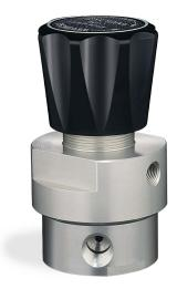
TESCOM DA Series absolute pressure reducing regulator is designed with an elastomeric diaphragm and provides accuracy to +/- 0.1 psig / 0.007 bar. This regulator may be used to reduce pressure from a supply source up to 4500 psig / 310 bar into a vacuum environment.
