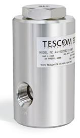
TESCOM 44-4200 Series is a high pressure, dome loaded, pressure reducing regulator with a  $C_V = 0.80$  or 2.0 available. This regulator is rated up to 6000 psig / 414 bar inlet and 5000 psig / 345 bar outlet.
