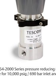
TESCOM 54-2000 Series pressure reducing regulator is suitable for 10,000 psig / 690 bar inlet and outlet hydraulic applications. Segregated and captured vent allows for convenient downstream pressure reduction adjustments. Hardened Stainless Steel seat and stem provide excellent wear resistance in harsh applications.
