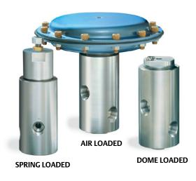
TESCOM 54-2200 Series pressure reducing regulator is designed for high flow and high pressure hydraulic applications. Inlet and outlet pressure is rated up to 8000 psig / 552 bar with  $C_V = 2.0$  for flows up to 60 GPM / 127 LPM. Spring, air and dome loaded versions are available. Hardened Stainless Steel seat and poppet delivers excellent wear resistance.
